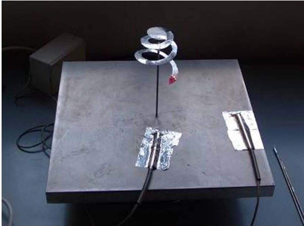
Fig. 3. Experimental apparatus: coil with 2 turns, thermometric probes and plate without lateral thermal insulation (photo taken in a non-operative stage).
